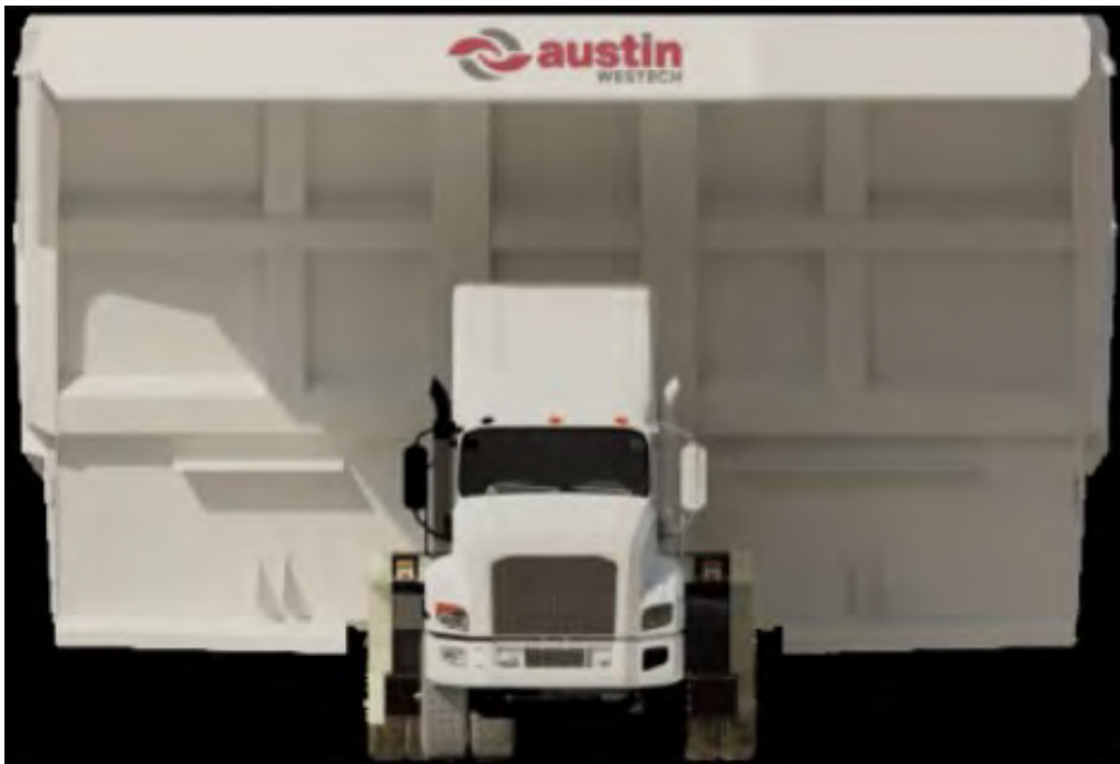
Figure 31 Westech Dump Body on Oversized Load Truck (35' maneuvering clearance)
